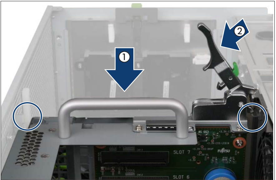
Figure 151: Installing the PCI Riser
